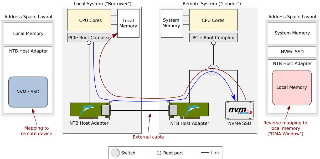
Figure 5: By mapping a remote device’s memory over an NTB, a local CPU may read from and write to it. Likewise, local system memory can be mapped for the remote device, allowing it to access local memory using DMA.
