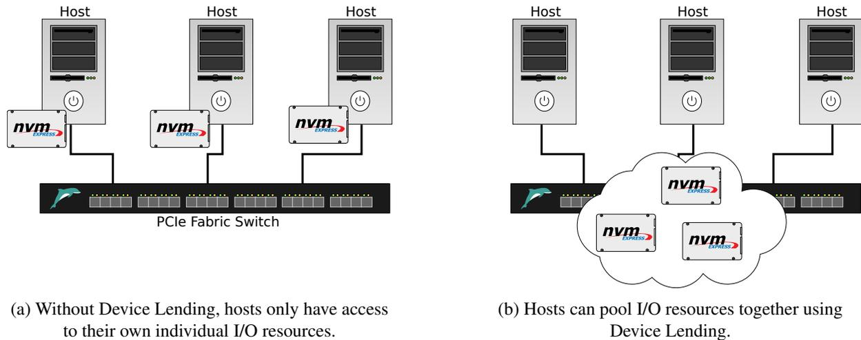
Figure 3: With Device Lending, devices become decoupled from the physical hosts they reside in. We can imagine this as connected hosts in a cluster contributing to a shared pool of I/O resources.
