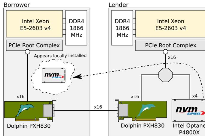
(b) Accessing a remote drive using Device Lending. As the drive appears local, the borrower uses the standard Linux NVMe driver to access it.
