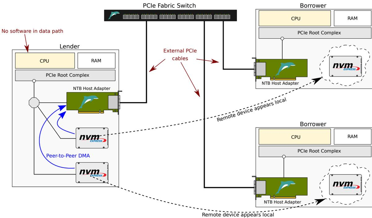
Figure 6: The Device Lending mechanism uses memory mappings to make remote devices appear as if they are installed locally. Since devices can be borrowed and returned dynamically, Device Lending is a highly flexible approach to composing the I/O infrastructure in PCIe clusters.
