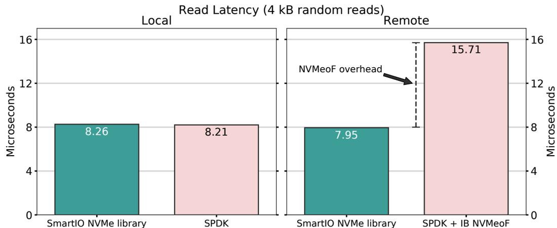
Figure 10: Results of our NVMeoF access latency comparison between SPDK and our SmartIO NVMe library. The FIO benchmarking program executed 327,680 reads of 4 kB each, using a random pattern. Note the overhead added by the NVMeoF protocol.
