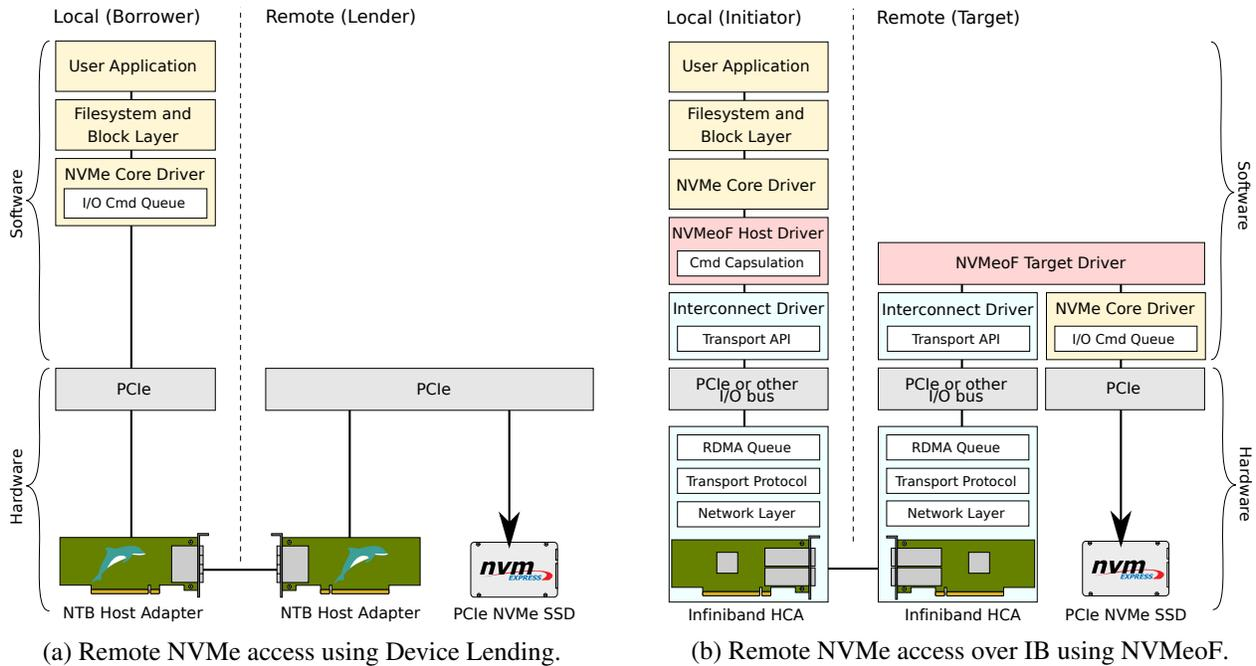
Figure 7: Device Lending makes the remote NVMe drive appear local, eliminating the need for forwarding I/O commands and RDMA transactions to the remote system. Instead, the local NVMe driver can access the drive directly over PCIe.
