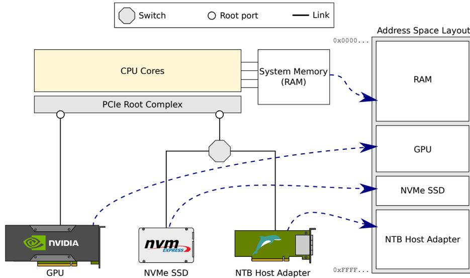
Figure 4: The system enumerates the PCIe device tree and maps device memory regions into the same address space as system memory. Devices that are capable of DMA can access system memory as well as other devices on the PCIe fabric.
