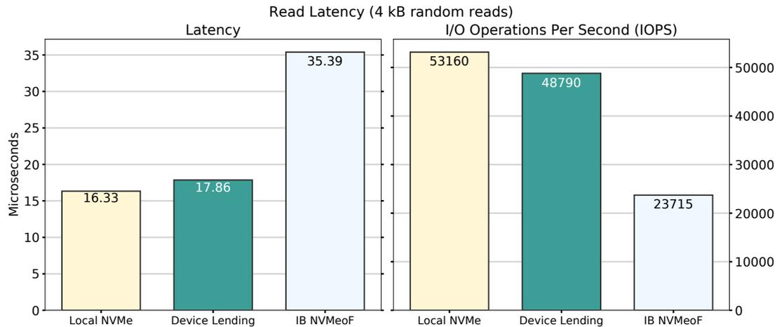
Figure 9: Results of our NVMeoF access latency benchmark using the Linux kernel driver stack. The benchmarking program executed 327,680 reads of 4 kB each, using a random pattern.
