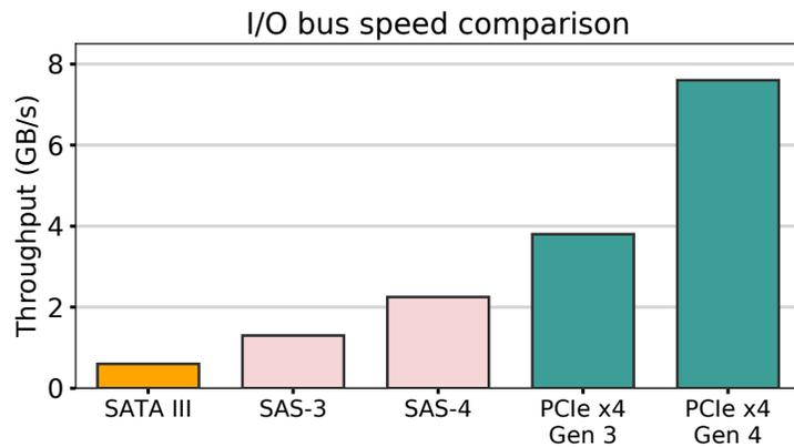
Figure 1: Throughput of PCIe compared to other traditional I/O buses. Consumer NVMe drives today are able to saturate a PCIe x4 bus for sequential reads.
