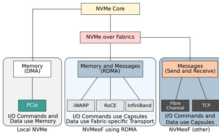
(a) Taxonomy of NVMe transport fabrics. Fabrics that support RDMA can provide very high performance compared to message-based transport.
