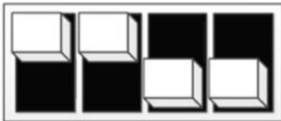
Illustration 7: SW1 – SWMODE - Default setting
