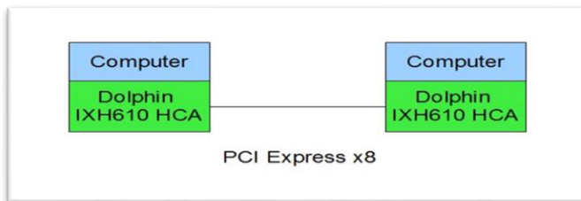
Illustration 4: Adapter card used to build a two node configuration.
