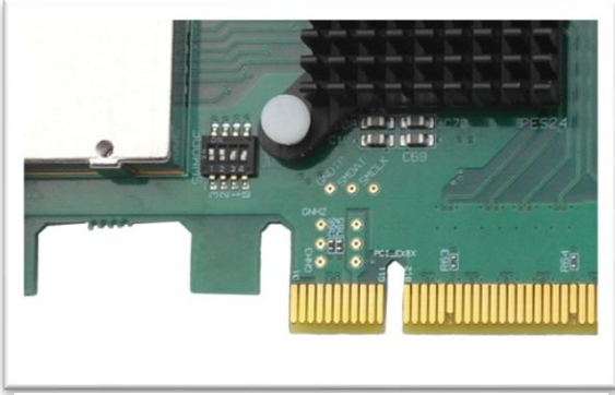
Picture 3: DIP Switch SW1 location
